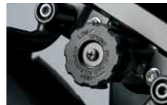
Useful spring preload adjustment
